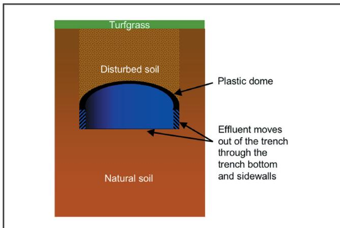
**Figure 3.** Cross-section of chamber trench.
