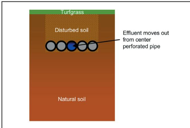
**Figure 5.** Cross-section of multiple pipe trench.
