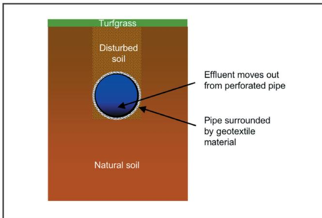
**Figure 6.** Cross-section of geotextile wrapped pipe trench.
