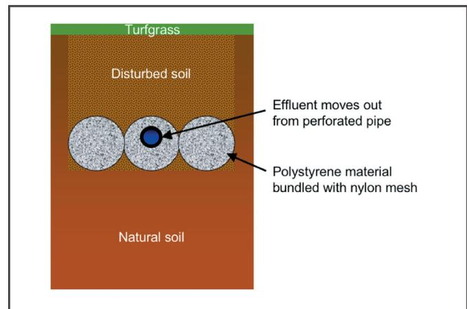
**Figure 4.** Cross-section of polystyrene trench.
