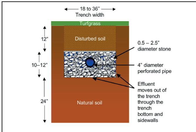
**Figure 2.** Cross-section of a conventional gravel trench. This trench is the most common type found in Indiana septic systems.
