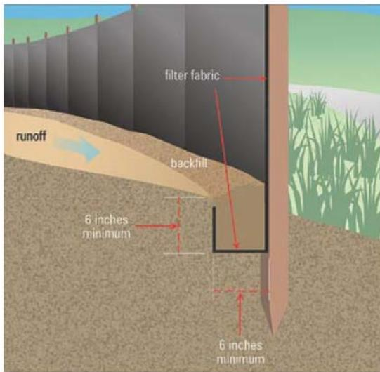
Install silt fence prior to land disturbing activities. Silt fencing should be installed 6 inches deep, at a minimum. Make sure wood stakes are on the downstream side of the flow.
