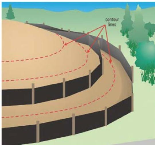
Install silt fencing along the contours. Make sure silt fence is spaced up the slope to allow for multiple ponding areas and to interrupt excessively long denuded areas.
