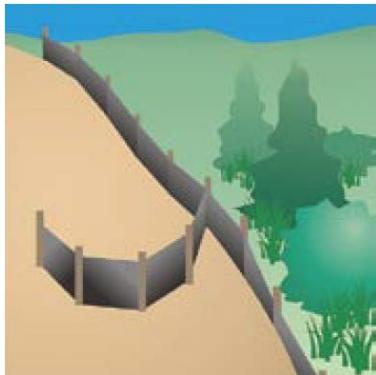
Install "J-hooks" along extended portions of diversion silt fence to promote ponding and minimize the potential for silt fence failure.
