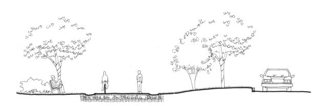
Figure 14: Section of Corridor with Multi-Use Path
