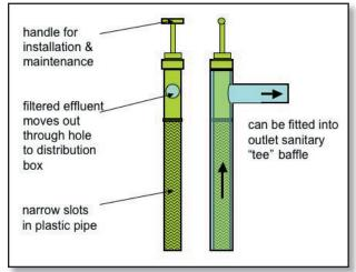
**Figure 3.** An effluent filter device is essentially a mesh screen that fits into or replaces the outlet baffle of the septic tank. It prevents solids from moving out of the septic tank and being deposited in the soil absorption field trenches.
