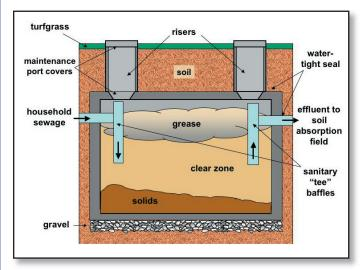
Figure 1. A cross-section view of a septic tank.
