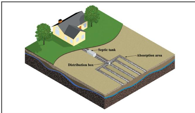
**Figure 1.** In a conventional trench septic system, wastewater flows from the house into the septic tank. In the tank, solids settle out and liquid waste flows into a distribution box, then through a network of perforated pipes placed in gravel filled trenches that are covered with soil. Collectively, this network of pipes is called the soil absorption field.
