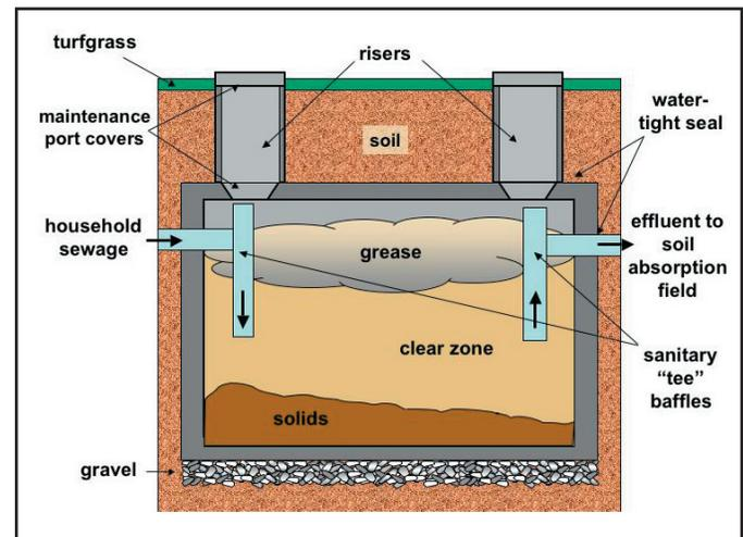
**Figure 1.** A cross-section view of a septic tank. Dense organic matter sinks while lighter wastewater components (grease and fats) float. The clarified effluent moves from the septic tank to the soil absorption field.
