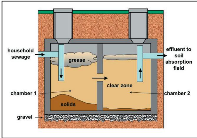
**Figure 2.** Dual chamber septic tanks help separate solids from the clarified effluent that will move out to the soil absorption field. These tanks require more frequent maintenance than comparably sized single chamber tanks.
