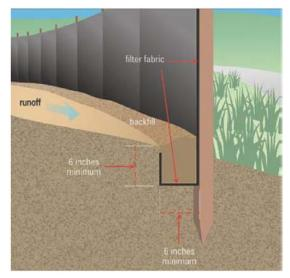
Install silt fence prior to land disturbing activities. Silt fencing should be installed 6 inches deep, at a minimum. Make sure wood stakes are on the downstream side of the flow.
