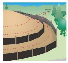
Install silt fencing along the contours. Make sure silt fence is spaced up the slope to allow for multiple ponding areas and to interrupt excessively long denuded areas.
