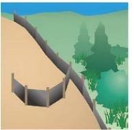
Install "J-hooks" along extended portions of diversion silt fence to promote ponding and minimize the potential for silt fence failure.
