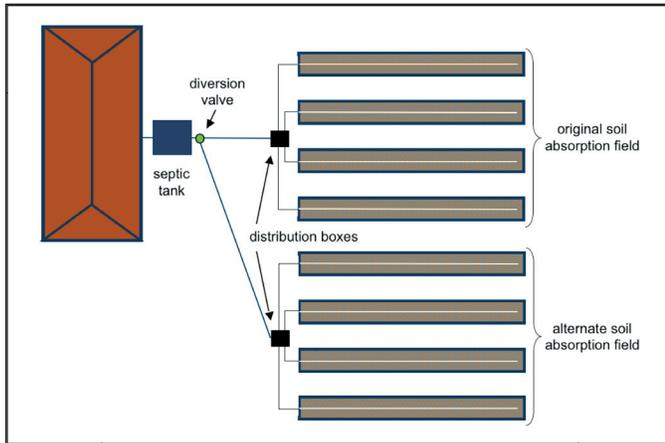
**Figure 2.** Alternating soil absorption fields are a common repair option for failing systems on larger lots. Diversion valves alternate the flow between soil absorption fields every six to 12 months. Resting a soil absorption field can restore a trench's infiltration capacity.
