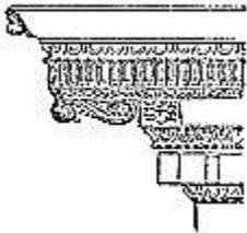
**Dentil** - is one of a series of closely spaced, rectangular blocks that form a molding. The dentil molding usually projects below the cornice, along the roofline of a building.
